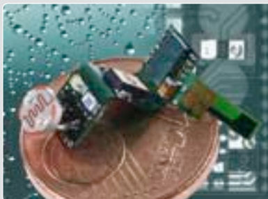
Worldwide smallest Sensor-Node with ad-hoc network capability (Mica-Z-Chipset)
