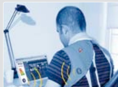
Detection of repetitive strain injury (RSI) with contactless capacitive EMG sensors (Courtesy of TNO)
