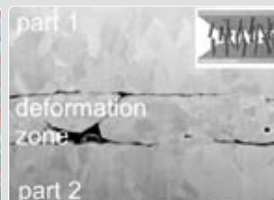
Cross section of joined Au-nanolawn @ 23°C, 100 mPa (bar: 1µm)
