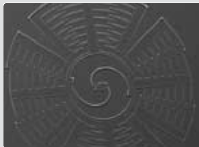
\mu -imprint of a sensor structure in PMMA
