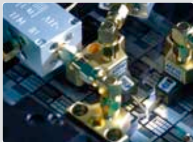
ATIS transient latch-up (TLU) module for sensitivity analysis at package and wafer level
