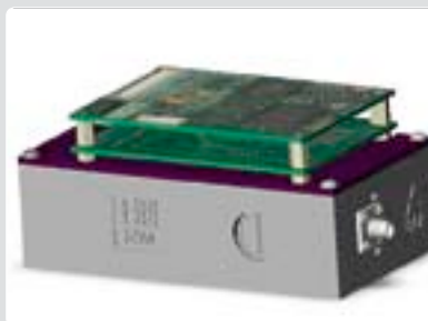
Schematic view of a MOEMS spectrometer for analysis in the near infrared range (NIR)
