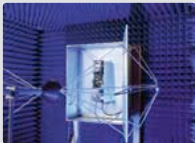
EMC test setup in the absorber chamber
