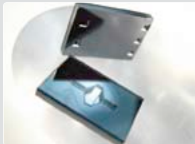
Bonded and diced MOEMS device (in cooperation with Ricoh Ltd. Japan)
