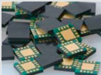
Transfer molded QFNs after singulation, ready for testing
