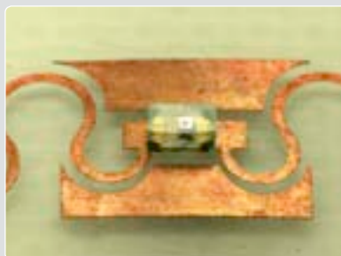
LED mounted to a stretchable substrate equipped with meandering Cu-tracks. The Cu structures surrounding the LED stiffen the substrate locally
