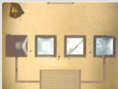
Self-assembled Si-Chips on copper pads
