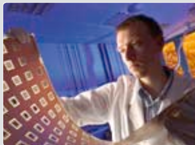
Embedding of thinned chips by vacuum lamination
