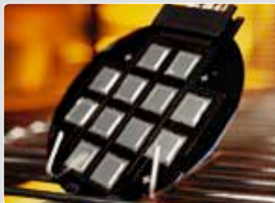
Encapsulated wafer-level battery on silicon oxide substrate
