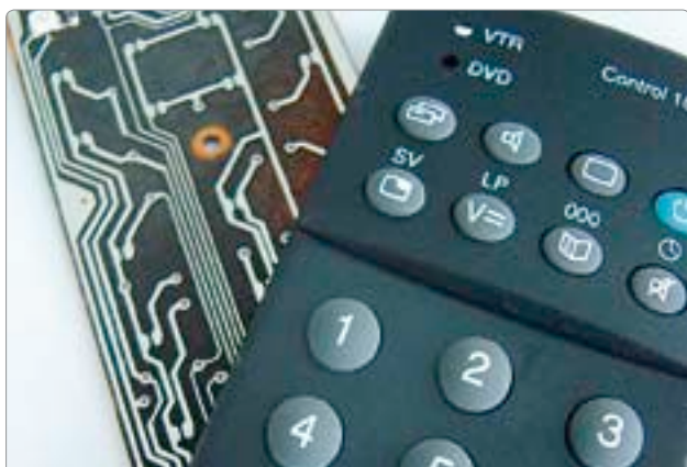
Printed circuit board for a remote control – based on lignin from wood or straw
